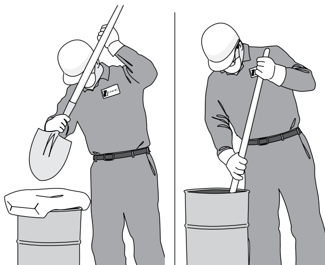
Figure 16 Mixing Slurry in Barrel
