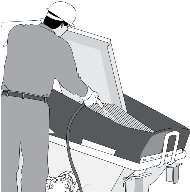
Figure 27 Clean Agitator and Hopper
