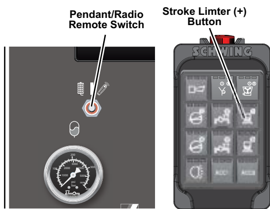
Figure 33 Pendant/Radio Remote Switch and Stroke Limiter Button
