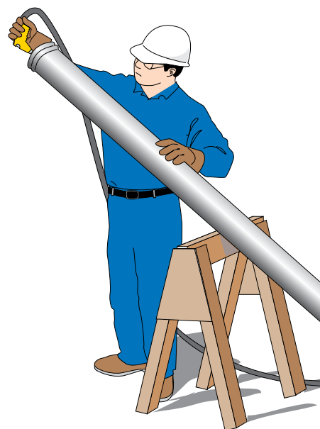
Figure 24 Washing the Pipe System
