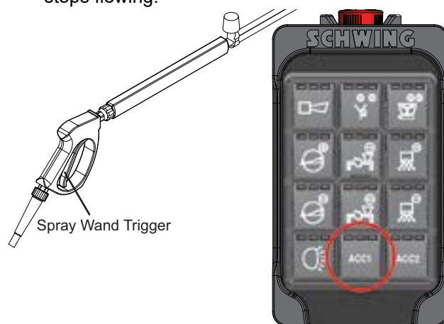
Figure 12 Spray Wand Trigger and ACC1 Button
