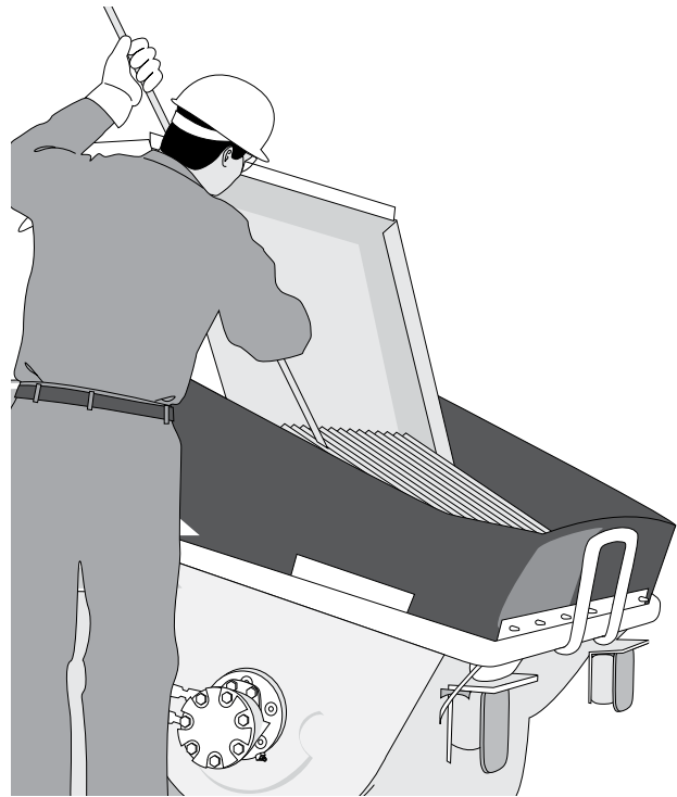
Figure 28 Remove Hardened Concrete From Hopper
