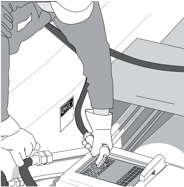
Figure 31 Spraying Out the Waterbox
