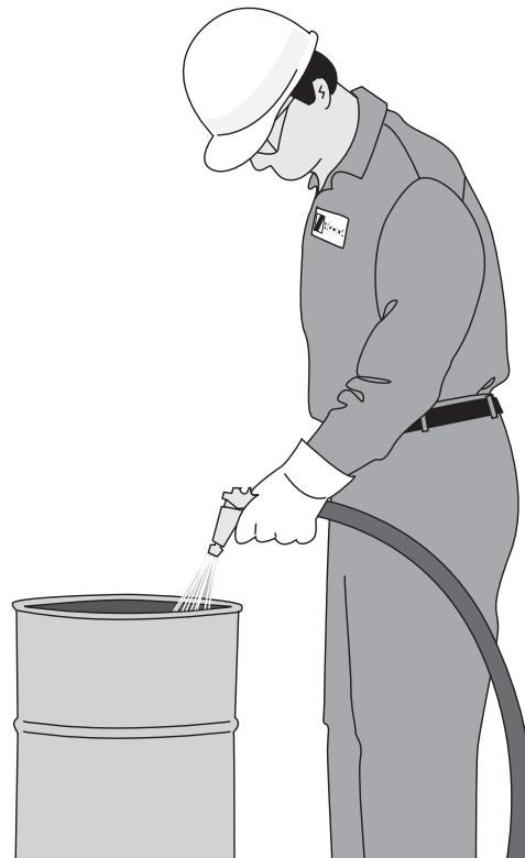
Figure 6 Water for Lubricating Slurry
