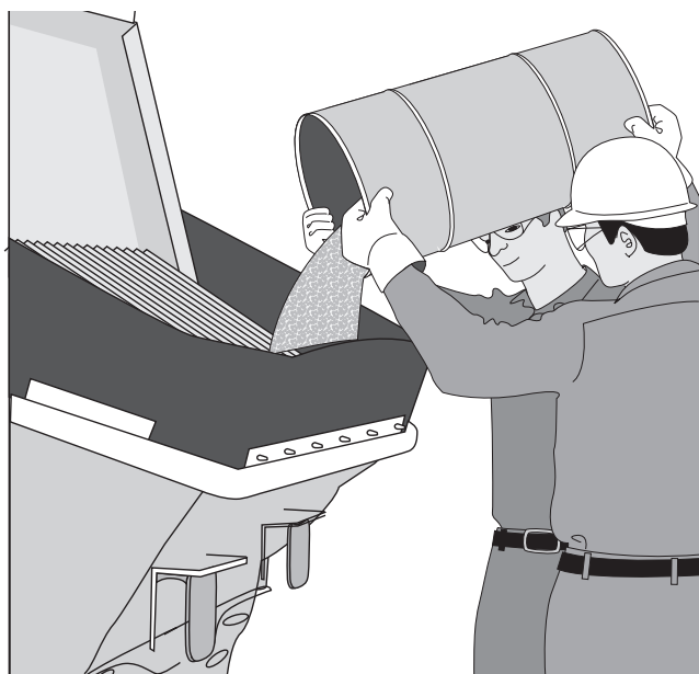
Figure 10 Pouring Slurry into Hopper
