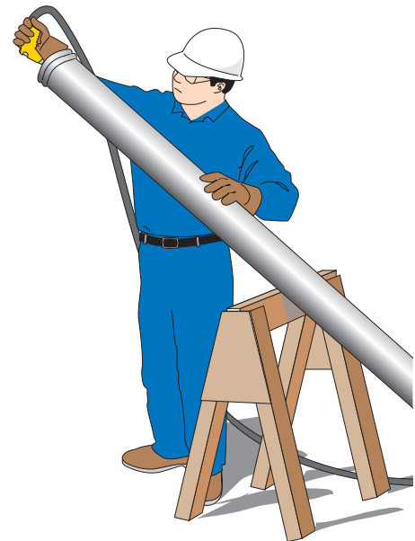
Figure 3 Washing the Pipe System
