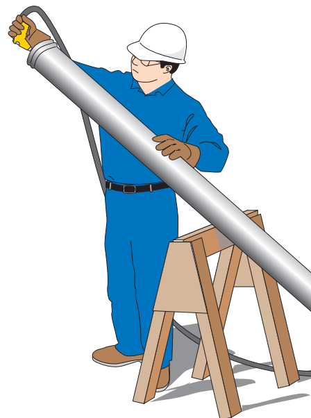
Figure 15 Washing the Pipe System
