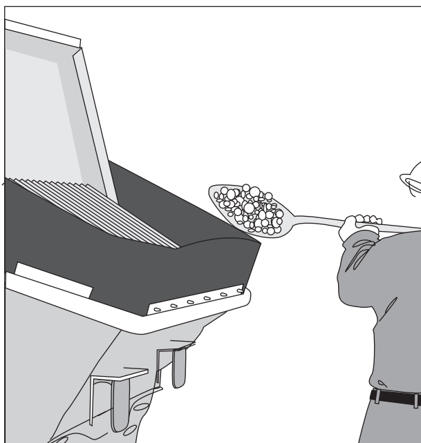
Figure 6 Sand to Cover Hopper Cleanout Door
