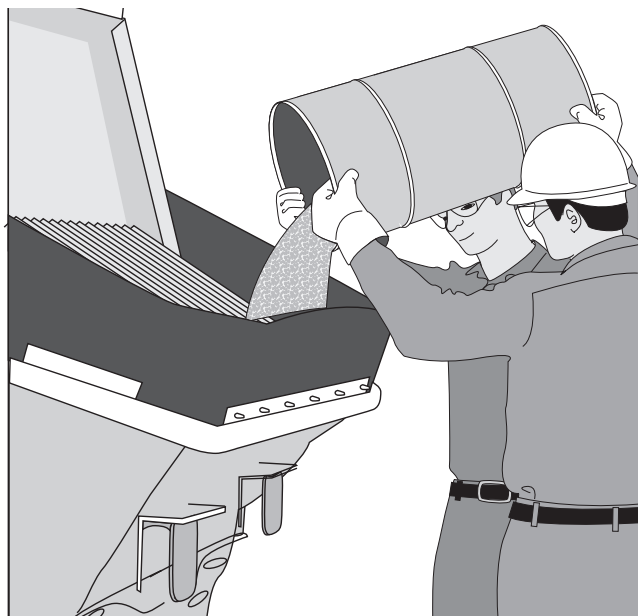
Figure 9 Pouring Slurry into Hopper
