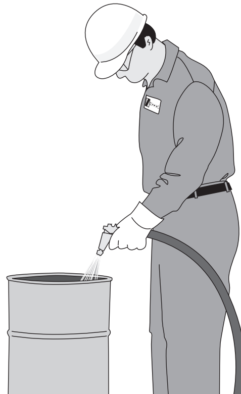
Figure 5 Water for Lubricating Slurry
