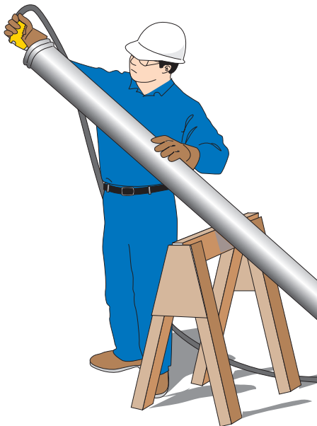
Figure 3 Washing the Pipe System
