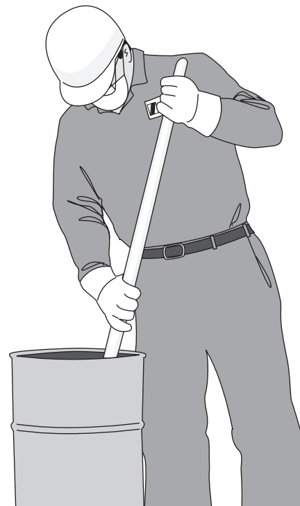
Figure 8 Mixing Slurry In Barrel
