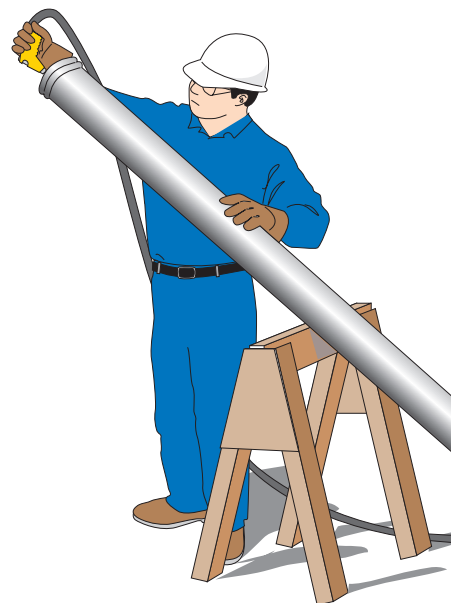
Figure 23 Washing the Pipe System
