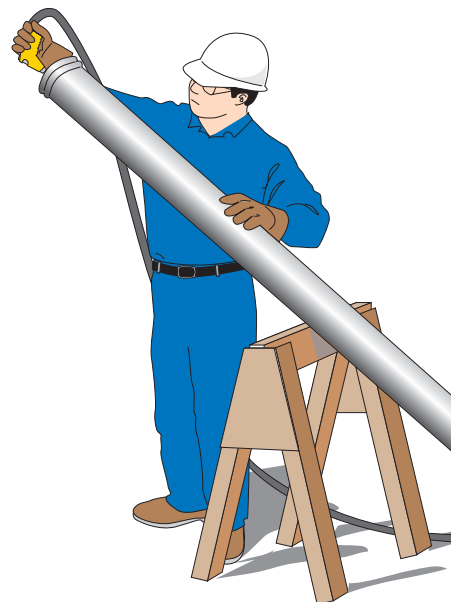
Figure 22 Washing the Pipe System
