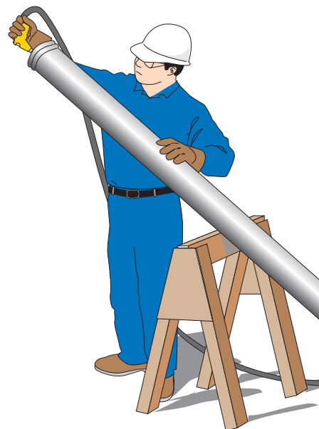
Figure 6 Washing the Pipe System
